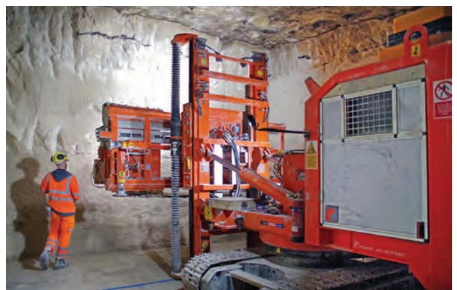
The cutting machine head carrying the chain saw can be traversed up/down; left/right and turned over
